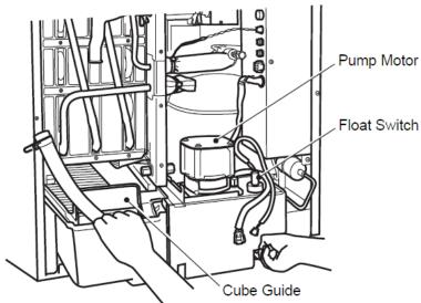
f. Remove the pump motor bracket securing the pump motor and the float switch. Remove the float switch from the pump motor bracket.
