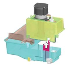
3) Flip over the pump motor bracket assembly, then twist off the float switch and pull out
