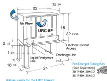
Voltage supply for the URC Remote Condenser is supplied from the Ice Maker No additional circuit is required.
